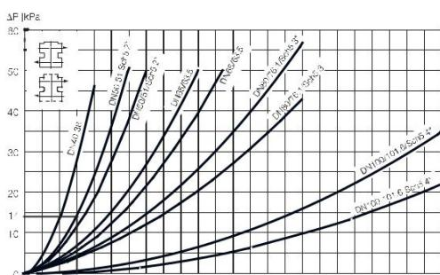
Pressure drop/capacity diagram, between bodies. 壓降/容量圖，在物體之間。
