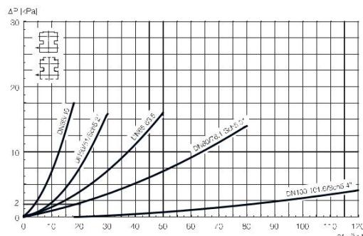
Pressure drop/capacity diagram, lower body, balanced and unbalanced lower plugs.
