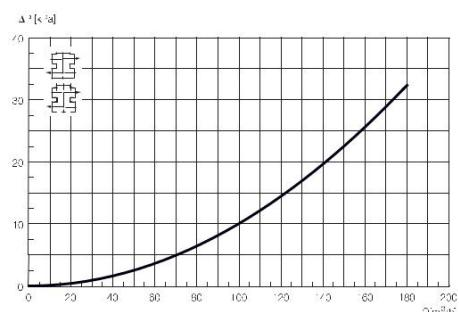
Pressure drop/capacity diagram between bodies Balanced and unbalanced plugs, DN 125, DN 150 平衡和不平衡插頭 , DN 125 , DN 150
