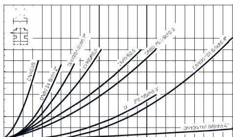
Pressure drop/capacity diagram, upper body. 壓降/容量圖，上體。
