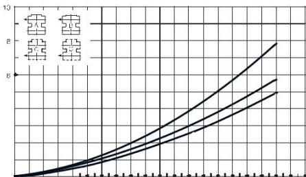
Pressure drop/capacity diagram, through bodies DN 125, DN 150 壓降/容量圖，通過閥體 DN 125 , DN 150
